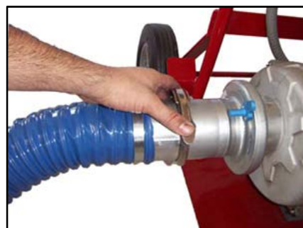
Fig. 6 – Hose Connect for Negative Duct Leakage Testing
