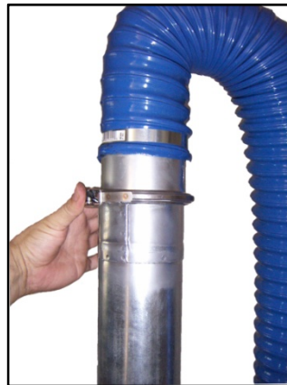
Fig. 5 – Hose Connection for Positive Duct Leakage Testing
