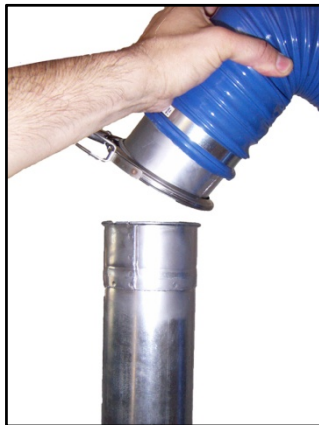
Fig. 5 – Hose Connection for Positive Duct Leakage Testing
